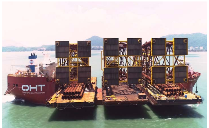
The team lowered transportation costs by 40% through the use of a single semi-submersible heavy-lift vessel instead of multiple tugboats.
